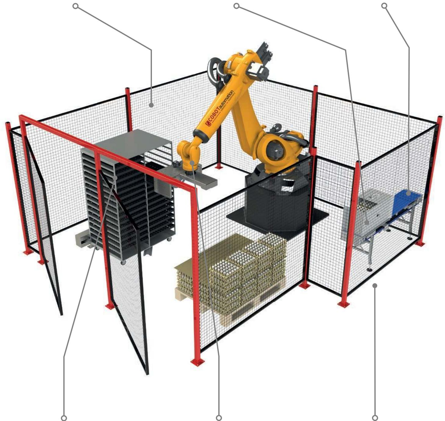
Robot automatically scans the exact shape and position of the setter tray in the container.
